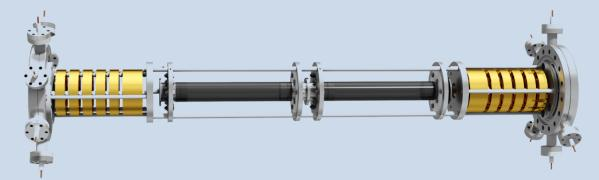
MR-ToF MS Trap for mass separation and mass measurements
