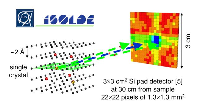
combined with radiotracer PL @ISOLDE for unambiguous correlation between structure and photonics
