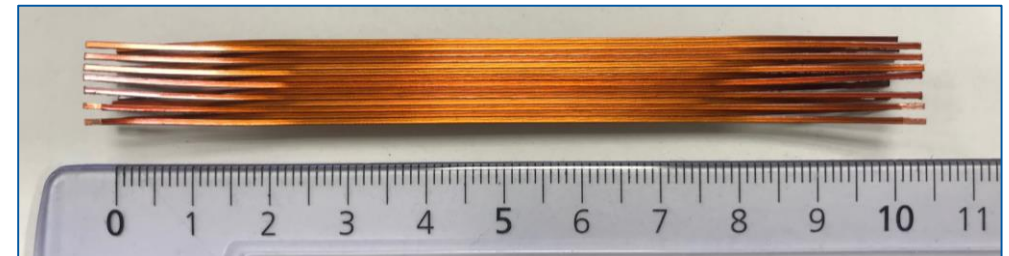
First non-valid sample. Short circuit at the ends.
