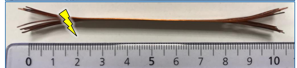
Second non-valid sample. The bending damages the insulation.
