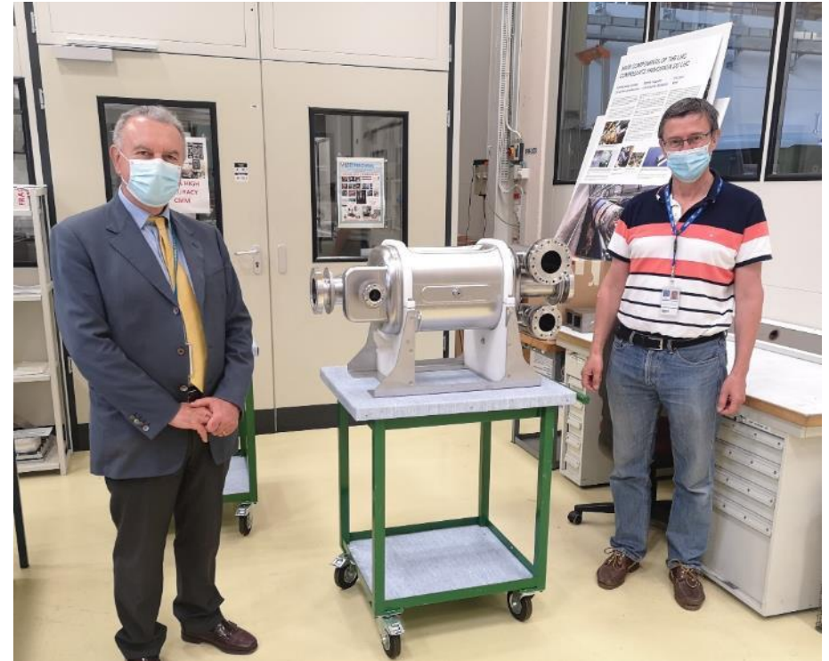
First RFD Crab cavity prototype (built at CERN) Ready to be tested and then completed with the helium vessel to be sent to UK (Daresbury) for completion with cryomodules. It will be the first RFD dipole completed and to be tested in SPS in 2022
