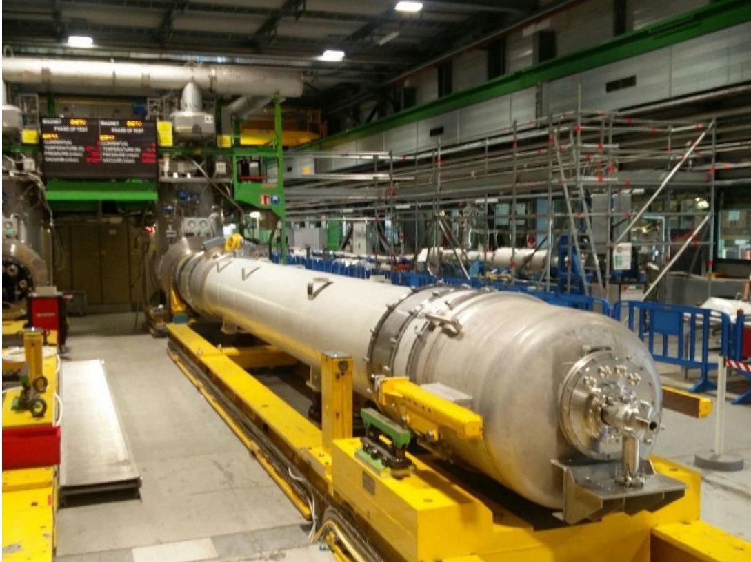
Inner triplet prototype MXQFB (coil length: 7.2 m) ready to be tested in SM18
