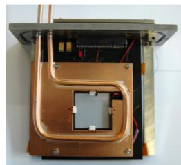
3×3 cm 2 cooled position- sensitive Si pad detector
