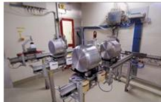
Clockwise from top left: Storage shelves for ISOLDE and CERN-MEDICIS targets after their operation, showing the robot for remote handling. A "fresh" target unit stands on the CERN-MEDICIS supply point, ready for the robot pick-up and transportation to the irradiation point. A rail conveyor system end-station for target transportation, showing the inspection camera and two modern target units. The MEDICIS building at CERN, next to ISOLDE. (Image credits: Yury Gavrikov.)
