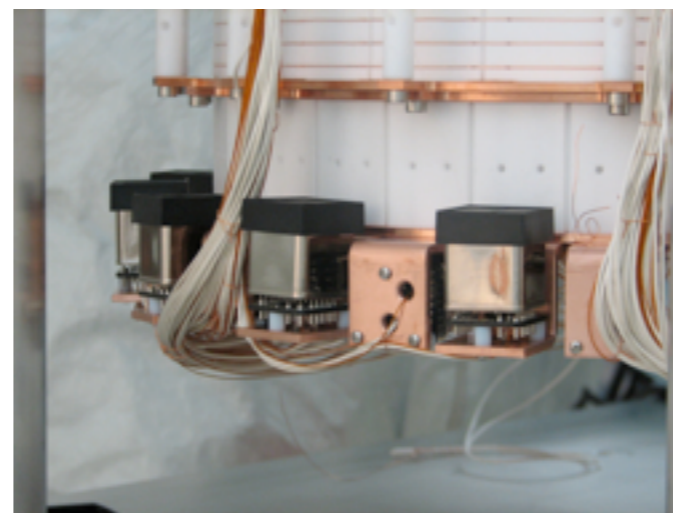
Top/Side Top arrays (32 PMTs)
