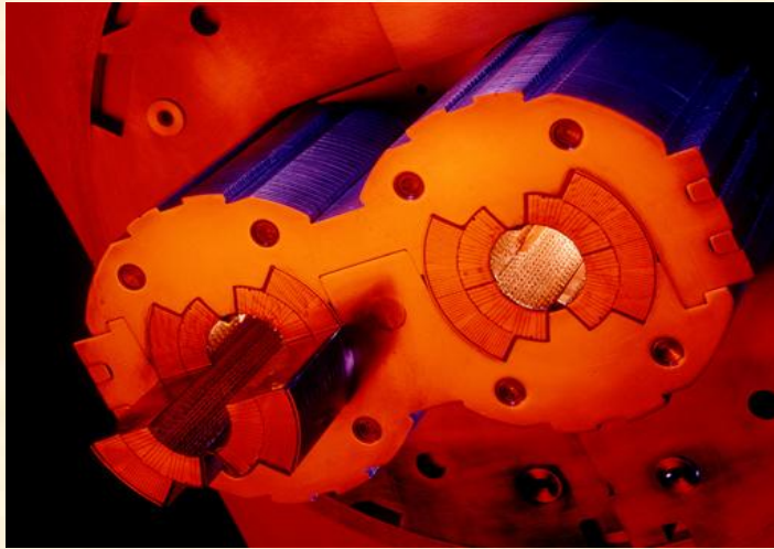
NbTi LHC standard dipoles, 8.3 T
