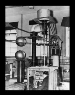
Proton accelerator used by Walton & Cockroft to split the atom. Walton sits in the small observation cabin and watches the produced alpha particles on a fluorescent screen. Credit: cambridgephysics.org
