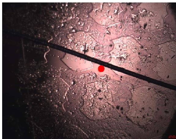
Picture 18: Semiconductor surface (black: wire with 60  $\mu\text{m}$ , red: beam spot of 50  $\mu\text{m}$ )
