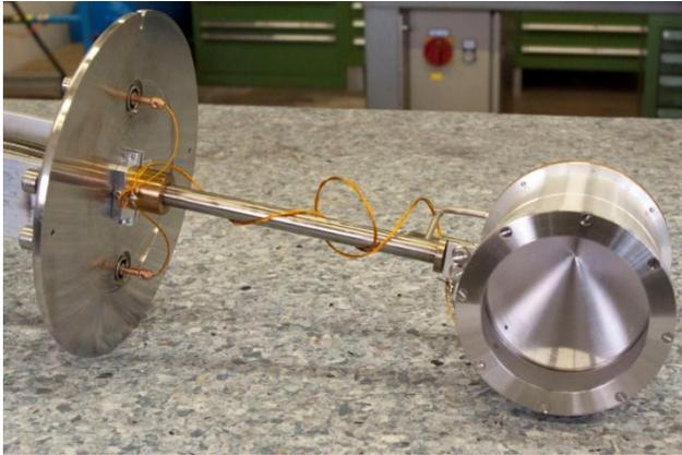
All other Faraday-cups have an opening of 25mm. Isolde counts 32 Faraday-cups and at the moment 9 are installed at Rex. Many of the 25mm Faraday-cups are
