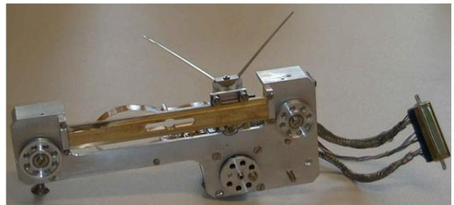
Most scanners at Isolde are x/y scanners. Equipped with a V-shaped pick-up (angle of 90°) the scanner chariot moves at 45° with respect to the horizontal plane thus producing both an x- and a y-scan of the beam profile. Originally equipped with pick-ups from Danfysik the pick-ups are now progressively being replaced by needles of material like that being used for medical syringes. The
