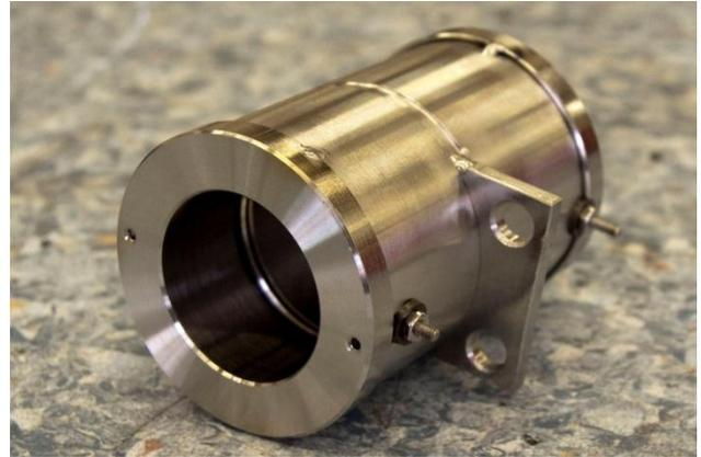
The repeller voltages used for the Faraday-cups vary from 130V for the small ones to 250V for the large ones.
