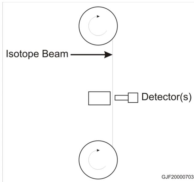
A Tape-station is very important at Isolde. Without it target and ion-source cannot be optimised which is equivalent to closing down the machine.
