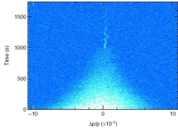
Figure 3: A sequence of Schottky spectra from a beam of  $Xe^{36+}$  ions showing the transition of the beam to an ordered state at around 1000 seconds.
