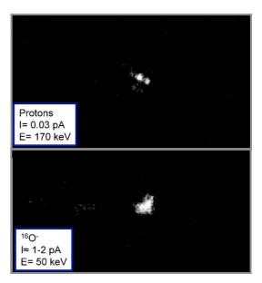
Fig. 11: sample images of very low energy and intensity proton and Oxygen beams detected by means of a CsI(Tl) screen and a CCD video camera. The spots are due to a pepperpot grid placed in front of the beam, the hole size is  $200\mu$ m.
