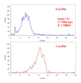
Fig. 6: example of X and Y beam profiles taken with plastic fibres, by counting particles at ultra-low beam intensity ( $\approx$ 7000pps <sup>s</sup>Li).
