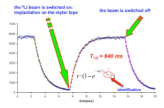
Fig. 9: identification of the <sup>8</sup>Li beam by means of its betadecay curve.
