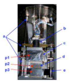
Fig. 8: the LEBI system for low energy and low intensity stable and radioactive beam imaging and identification. Shown are: (a) the tape transport system; (b) photomultiplier; (c) the plastic scintillator; (d) the CsI(Tl) plate; (e) the Mylar tape. The system can be positioned in beam into three measuring positions: (p1) beam rate measurement; (p2) imaging of stable (pilot) beams; (p3) imaging of radioactive beams.
