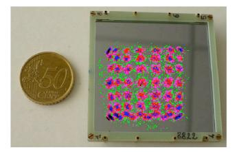
Fig. 2: a  $5x5cm^2$  position sensitive silicon detector. Superimposed to the picture one can see the linearized plot obtained after sending the beam on the sensor across a pepperpot mask.
