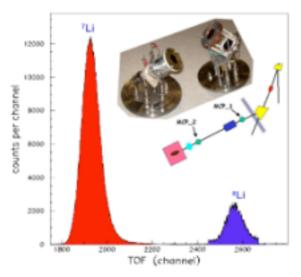
Fig. 4: example of Time Of Flight technique for online identification and tagging of the <sup>8</sup>Li radioactive beam by means of two MCPs detecting secondary electrons emitted by a thin carbon foil.
