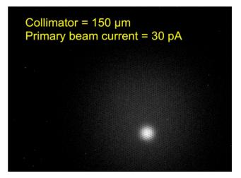
Fig. 7: transverse profile of a low intensity proton beam after collimating it to  $150\mu$ m diameter. The primary current was 30pA.
