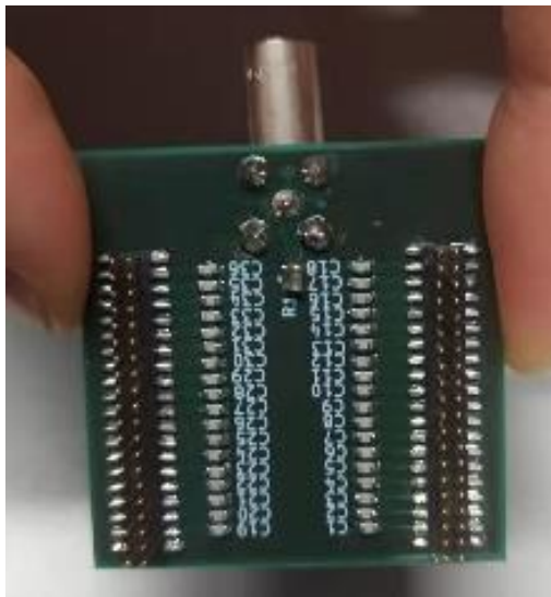
Adapter PCB to inject charge pulses injection to 36 channels
