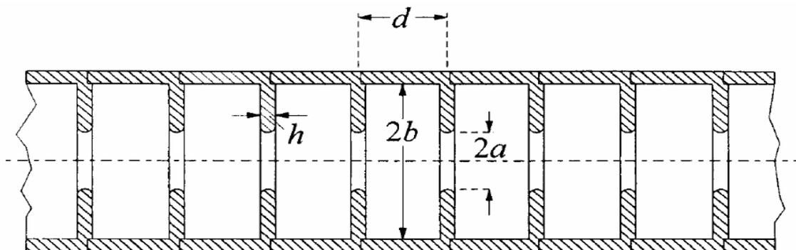
Assuming that the cavities are operated in the  $2\pi/3$  mode with a phase velocity  $\beta_z = 1$  and a supplied power of 35 MW, what is the total accelerating voltage and energy gain per metre for a SLAC structure of length  $l = 3$  m.?
