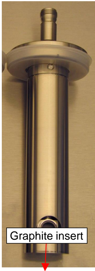
Flange mounted, 4W beam power
