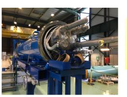
Crucial milestone: first Nb<sub>3</sub>Sn dipole (left) and inner triplet quadrupole (right) for HL-LHC built and qualified for installation at CERN and in the US.
