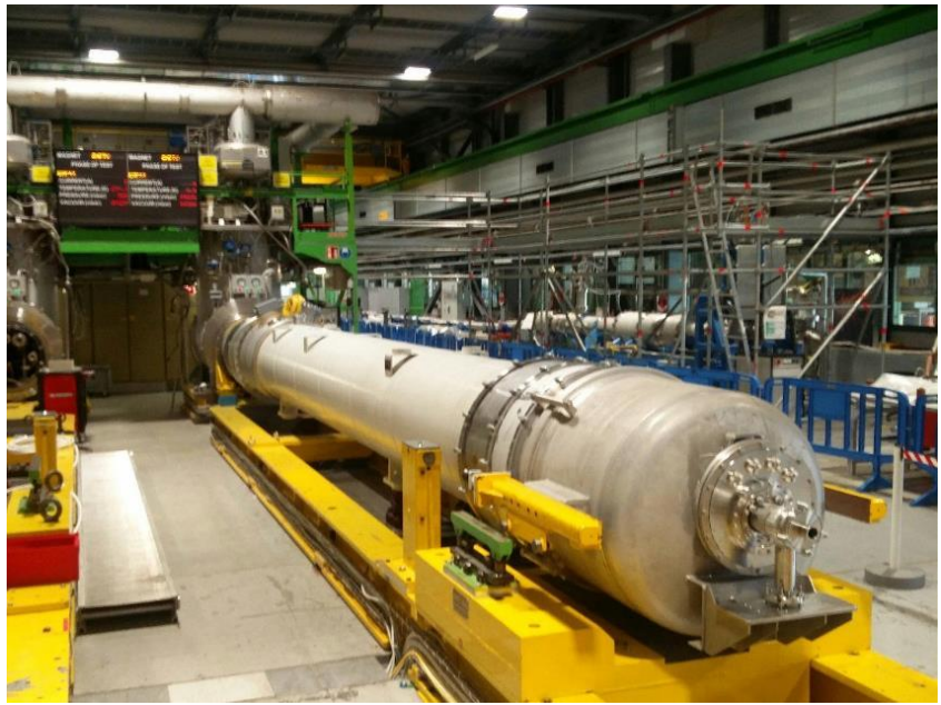
Nb 3 Sn inner triplet full-size prototype (7.2 m) ready to be tested in SM18
