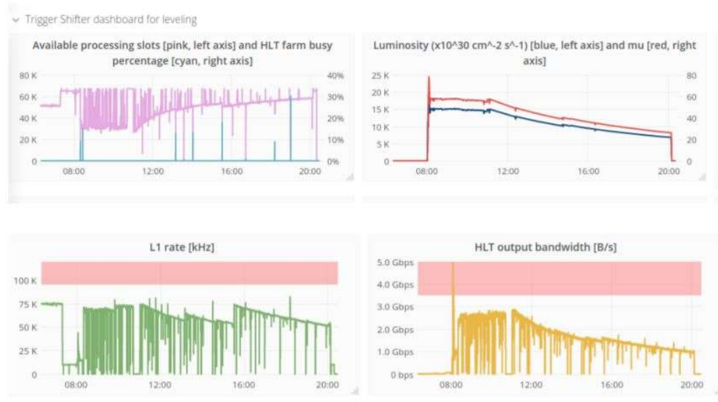
Figure 18: An example of a P-BEAST dashboard as used by the shifters during 2017 operation. The HLT farm availability (top left), the luminosity and the pileup, “mu” (top right), the total L1 accept rate (bottom left), and the total HLT output bandwidth (bottom right) are shown.
