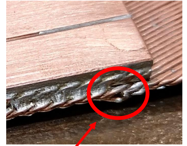
Broken strand on a cable edge
