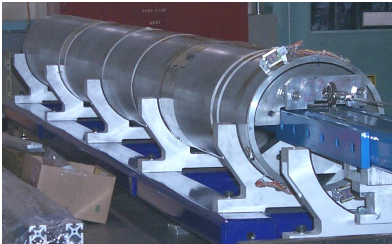
Structure re-assembly with segmented shell
