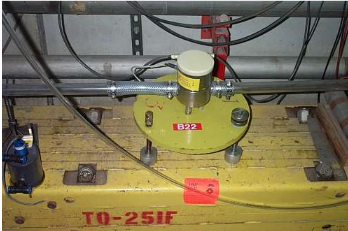
Fig.35. HLS probe on Tevatron accelerator focusing magnet.
