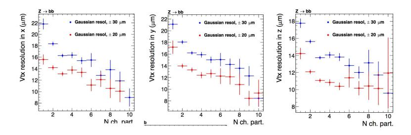
Resolutions:  $\sigma(x, y)^{15}\mu m$ ,  $\sigma(z)^{12}\mu m$
