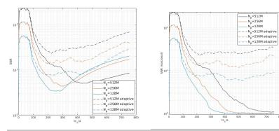
Noise leads to increased shearing rate, which in turn suppresses turbulence:
