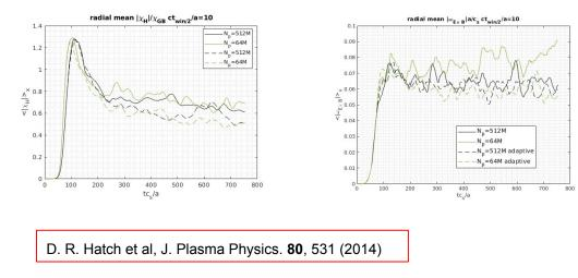
Simulations are less sensitive to marker numbers in general, but shearing rate increases when marker number decreases
