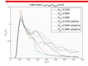
Non-adaptive case: Drop in heat flux and diffusitivity due to noise, leading to negligible residual values
