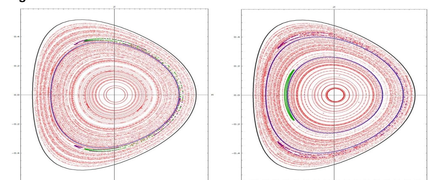
which appear in certain rational magnetic surfaces. That happens because a magnetic island has necessarily a rational safety factor, otherwise it would never be closed to itself. For illustration purposes we highlight a large island appearing at the q=1/6 surface of the m=6 equilibrium (left) and two islands that appear at q = 1/8 and q = 2/8 surfaces of the m = 8 equilibrium (right).
