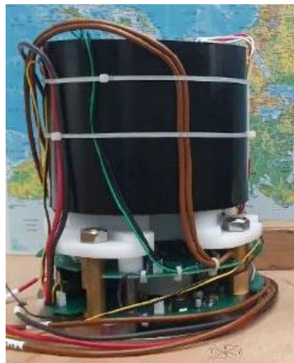
Figure 1: the new AC/DC converter
