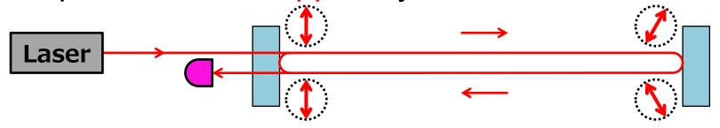
Bow-tie cavity can amplify the rotation
