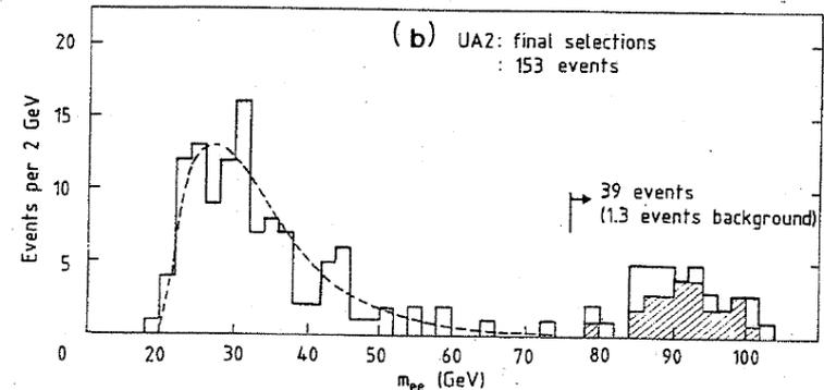
Figure 12.5: (a) The invariant mass distribution for  $e^+e^-$  pairs identified through electromagnetic calorimetry in the UA-1 detector. (Figure supplied by UA-1 Collaboration) (b) The analogous plot for the UA-2 data (Ref. 12.12). In both data sets, the  $Z$  appears well-separated from the lower mass background.
