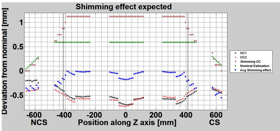
Fig. 5. Additional shims to achieve nominal pre-compression of outer dipole coils in first prototype. Vertical lines show the pole window length.
