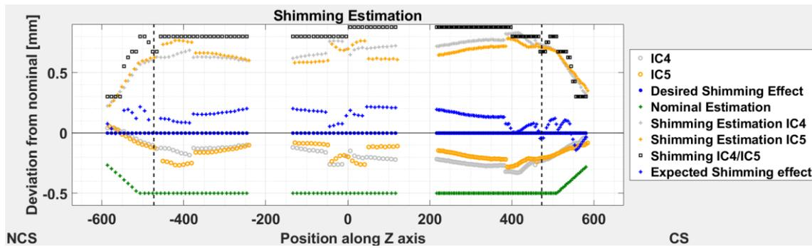
Fig. 8. Shimming proposal for inner dipole coils of second prototype.
