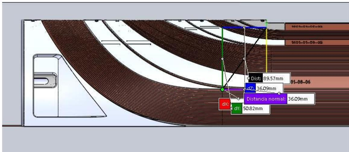
Fig. 3. Inner dipole coil end: the midplane block cables of the outer layer are 36 mm longer than the coil pole window.
