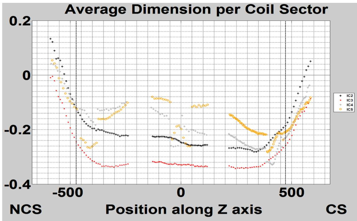
Fig. 1. Average deviation (mm) from nominal coil arc length along its longitudinal axis.
