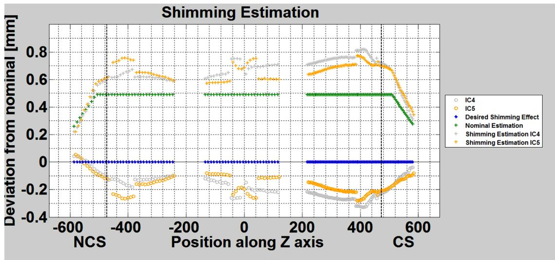
Fig. 7. Estimation of additional shims for inner dipole coils of second prototype.
