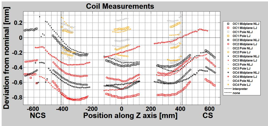
Fig. 4. Measurements of the arc length of the outer dipole coils: OC1 and OC2 were assembled in the first prototype, while OC3 and OC4 will be assembled in the second prototype.
