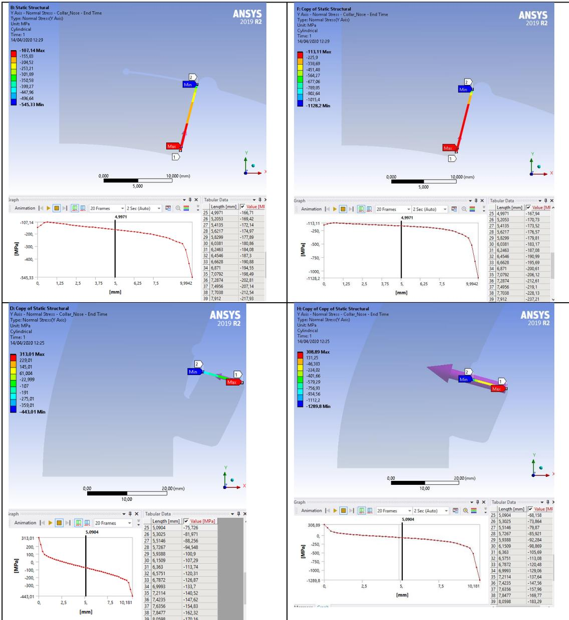
Fig. 6. Above, both inner dipole collars (instrumented and non-instrumented) feels the same pre-load. However, outer dipole instrumented collars (bottom left) feels about 10% more stress than non-instrumented ones.
