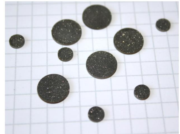
Figure 4 Diamond-Ti luminescent screens (a) before hotpressing (b) depth profile of embedded diamonds (c) samples extracted from larger hotpressed sample
