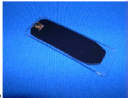
Fig.5 a) printed circuits boards were used as main MRPC structure on which copper strips or pads were engraved; b) standard microscope analysis glasses were used for the external electrodes; a semi conductive adhesive tape was used as HV and ground distribution.
