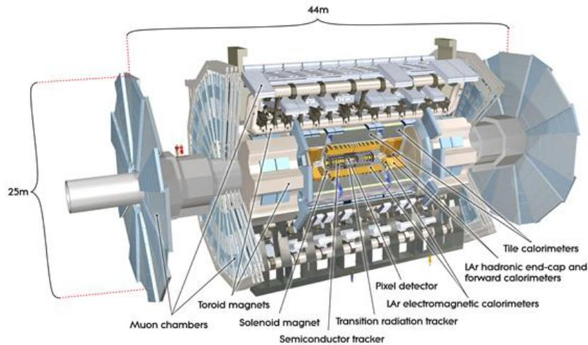
**Figure 1.** The ATLAS detector and its subsystems (extracted from CERN Document Server CERN-GE-0803012 01).
