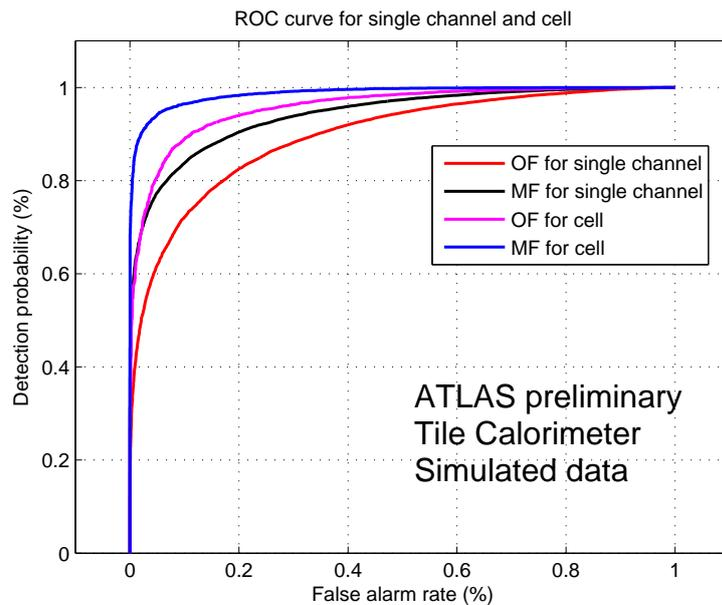
**Figure 7.** Detection efficiency against false alarm rate for all four analysis.
