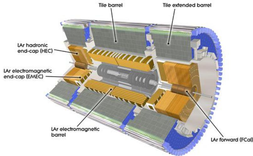
**Figure 2.** The ATLAS calorimetry system (extracted from CERN Document Server CERN-GE-0803015 01).
