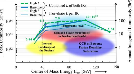
Recent machine development and studies Possible to get high luminosity by only adjusting magnetic polarities of near-IR magnets
