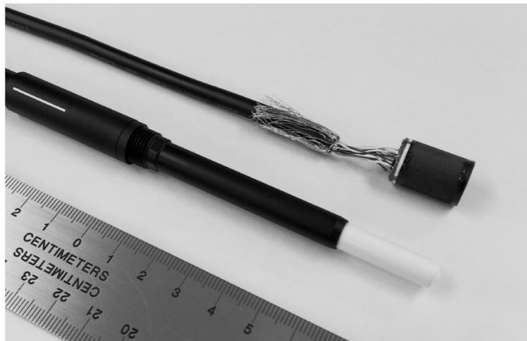
A prototype without its waterproof housing, next to a SNC 600c Farmer chamber
