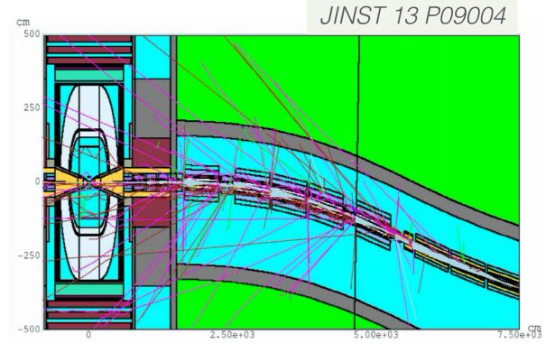
interaction of secondary electrons with the whole accelerator have been simulated with MARS15 and transported to the detector for further simulation
