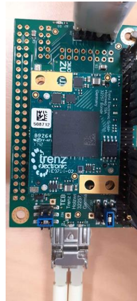
Artix 7 GTP receiver used for interoperability tests with OSERDESE3 sender
