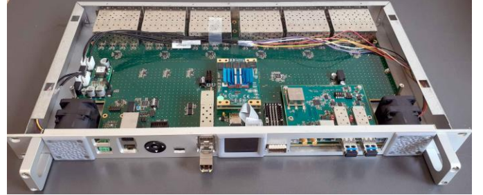
Fig. 3. Prototype 48-port clock distributor board.
