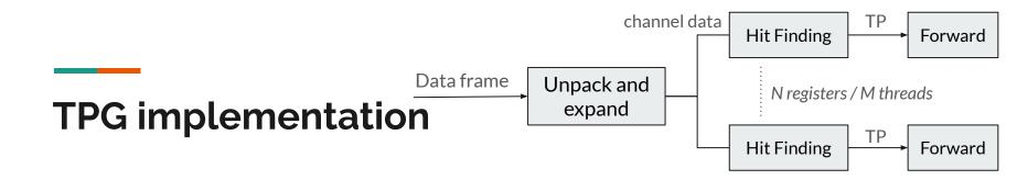
Single instruction Multiple Data (SiMD) parallelized implementation with the use of <u>Advanced Vector Extensions (AVX)</u> to the x86 instruction set. Use of AVX2 registers with 256 bits. The TPG chain consist of:
