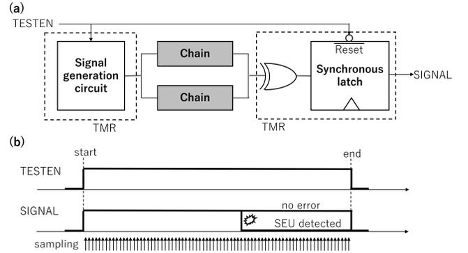
Fig. 4. (a) Schematic view of the evaluation circuit for SEU on the AS-FPGA, and (b) the timing structure of SEU detection.
