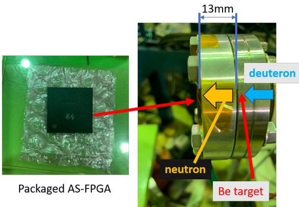
Fig. 3. Photograph of the packaged AS-FPGA and the experimental setup for neutron irradiation test.
