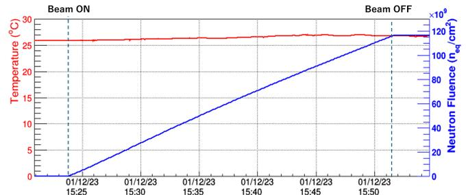
Fig. 11. Obtained temperature data from the newly developed slow-control board (red) and neutron fluence (blue).
