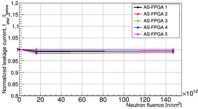
Fig. 5. The leakage currents for 5 AS-FPGA chips before and after neutron irradiation.
