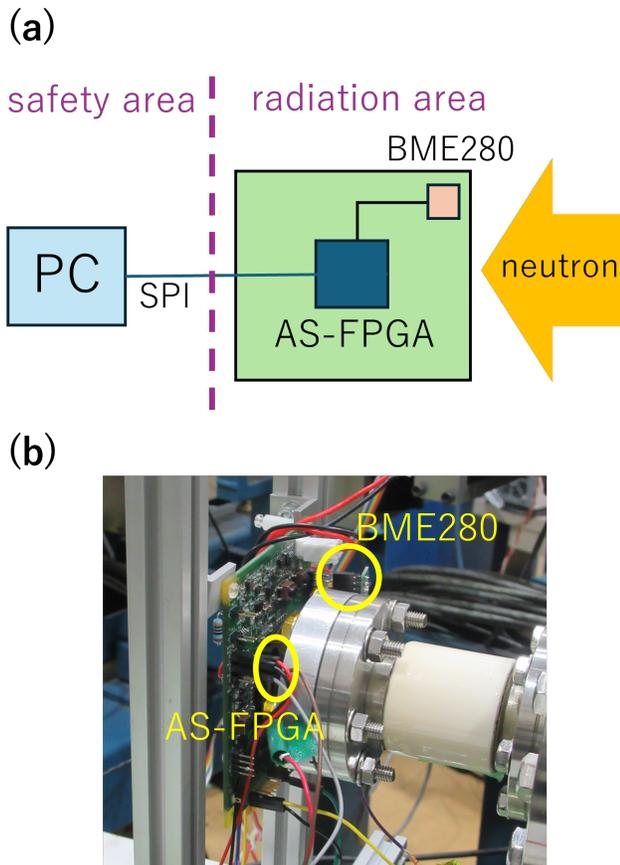
Fig. 10. (a) Schematic view of the experimental setup for the neutron irradiation test of the newly developed slow-control board. (b) Photograph of the experimental setup. The center of the slow-control board was set at the beam center, 20 mm from the Be target.
