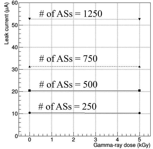
Fig. 6. The leakage currents for AS-FPGA chips before and after gamma-ray irradiation.
