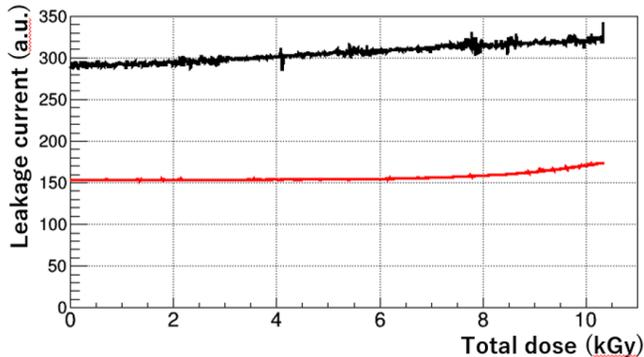
Fig. 8. Leakage currents during gamma-ray irradiation for the AS-FPGA (red) and the LP-FPGA (black).
