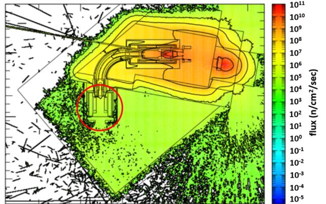
Fig. 1. Radiation level of neutrons for COMET Phase-I calculated with PHITS. Red circle shows the region for detector and front-end electronics.
