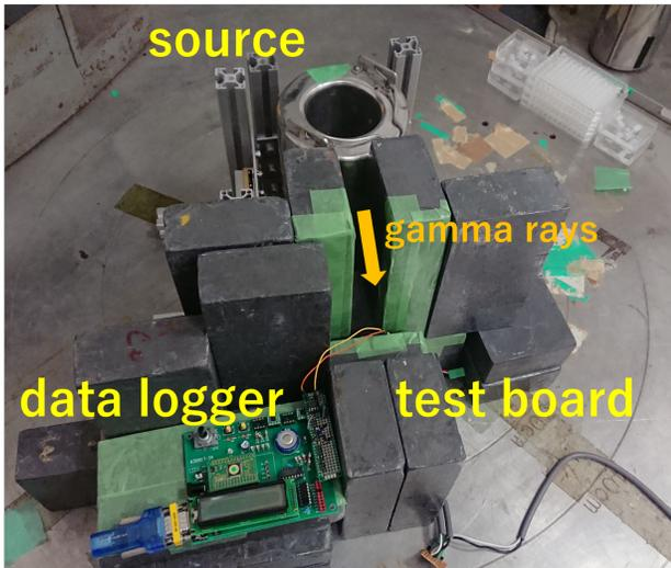
Fig. 7. Photograph of the experimental setup of gamma-ray irradiation for AS-FPGA at TITech.
