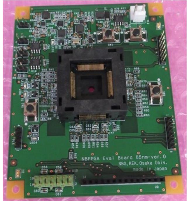
Fig. 9. Photograph of the evaluation board for the AS-FPGA.
