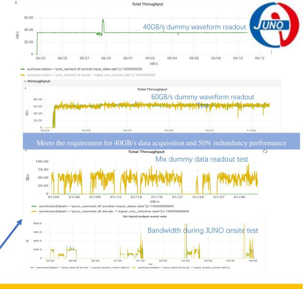
The current version of JUNO data flow software supports readout and processing of waveform and T/Q data for both CD and WP detectors, as well as global trigger data. The on-site detector integration has begun, and the software is currently able to support trial operation.
