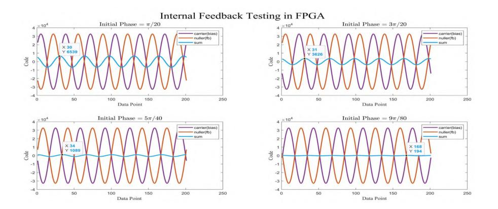
The bias signal and feedback signal are sent to the adder, then they are connected to the ADC. Both the amplitude and phase need to be adjusted.
