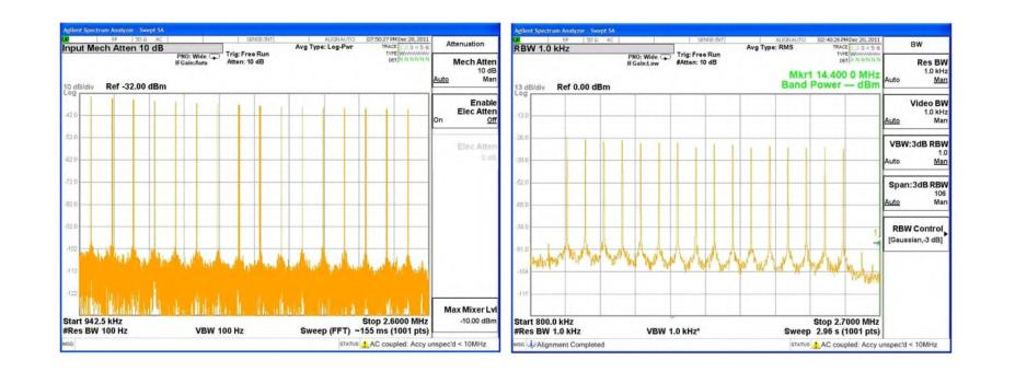
In order to make the test more accurate, we limited the range of the spectrum chart to around 1.8M. The signal-noise ratio (SNR) is about 80dBc.
