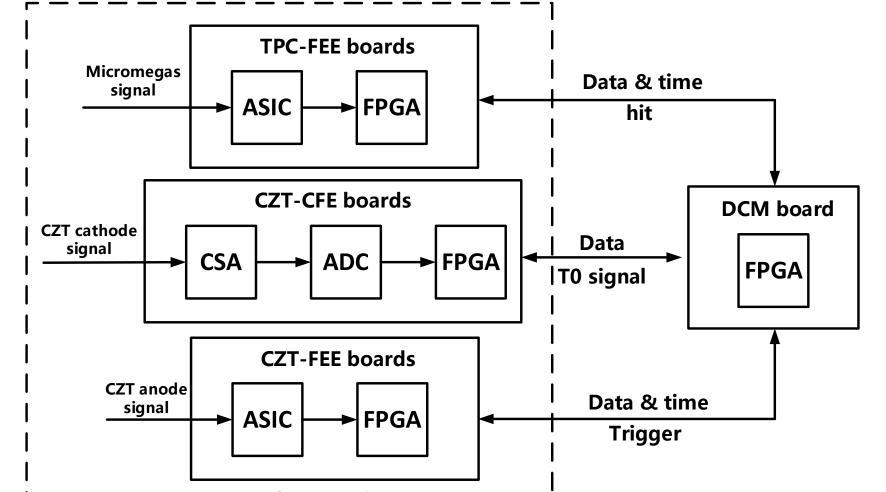
The TPC anode electronics require multi-channel CSAs to integrate charge from the TPC anode. It is necessary to obtain the original waveforms of TPC anode signals with the ASIC. Thus we can identify the signals by waveform analysis when two groups of electrons drift to the same strip successively. The front-end electronics includes following parts:
