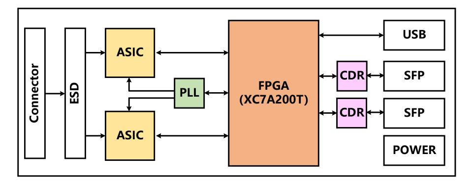
CZT anode electronics require multi-channel, lownoise CSAs. A 64-channel low-noise ASIC named VATA453 is chosen, which was developed by IDEAS. Each channel of the VATA453 chip has:
