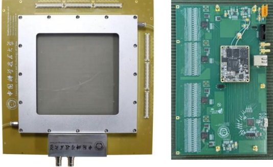
Fig. 3. Micromegas Detector and the front-end electronics board.
