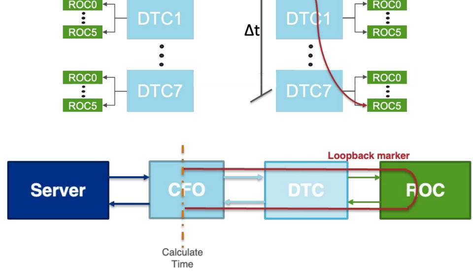
High level configuration of the pre-production TDAQ system deployed at the Mu2e Experimental Hall. DTCs collect data from sub detector ROCs, perform event building, and data processing.
