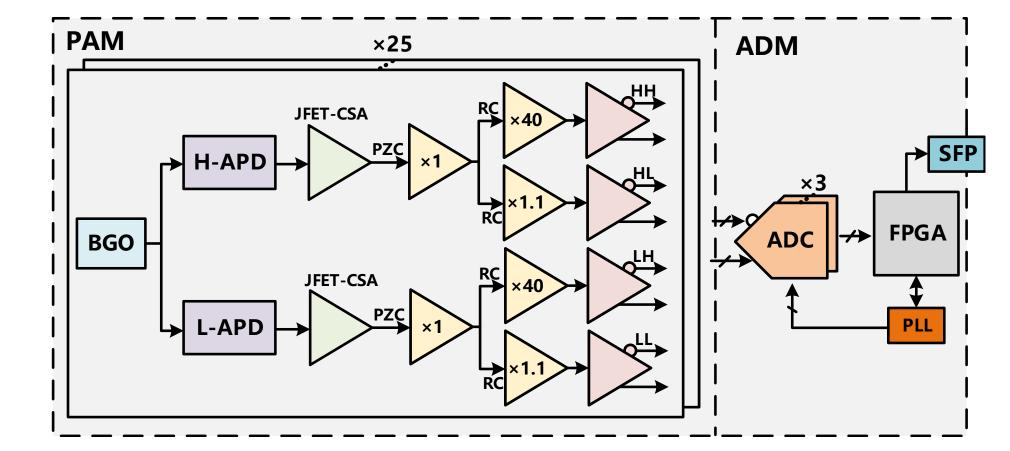
For an APD, the readout electronic dynamic range can reach from 3 fC to 7 pC.
