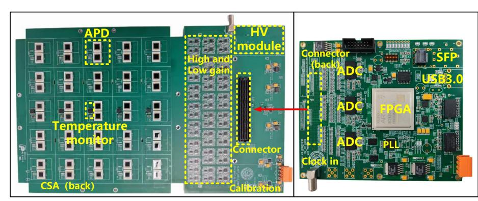
Measuring cosmic rays using a self-triggering mode: When a crystal within the calorimeter is hit by a cosmic-ray, ADM sends a hit signal to the DCM. Then the DCM issues a trigger signal to receive the waveform or amplitude data of the current event.
