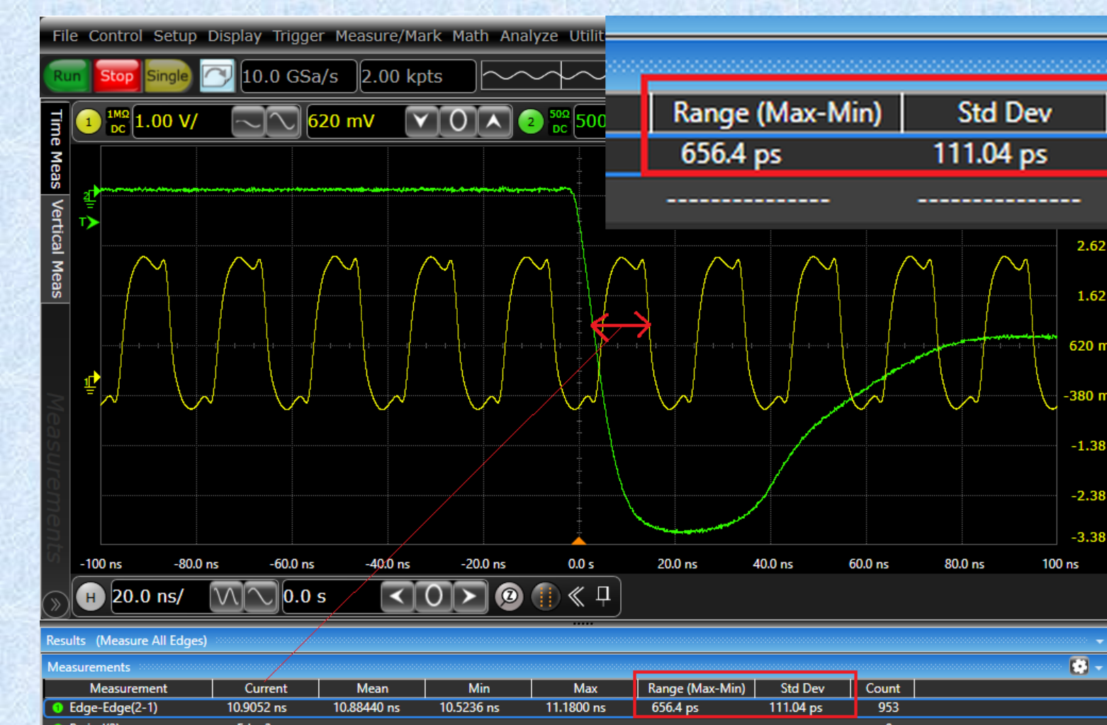
Figure 7: Clock jitter measurement. Yellow: clock on TTCL interface board, green: trigger from TTCL master.
