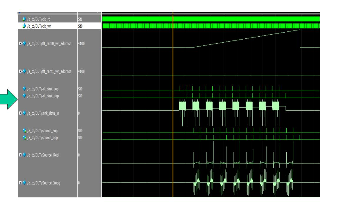
Real-time MHD system on KSTAR computed real-time FFTs from the toroidal magnetics probes for the first time in 2021 for real-time DECAF application.
