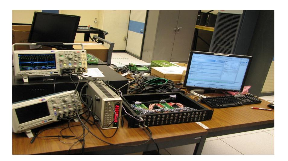
When constructing the FFT engine in hardware, Intel FFT IP core is used to implement FFT. The detailed pipelining and timing for 16 channel 512 sample points for the FFT engine is described in the paper. Dual FIFO and RAM ping pong architecture are used for data reading, processing, and writing. The test result shows that the pipelined FFT engine works as expected.
