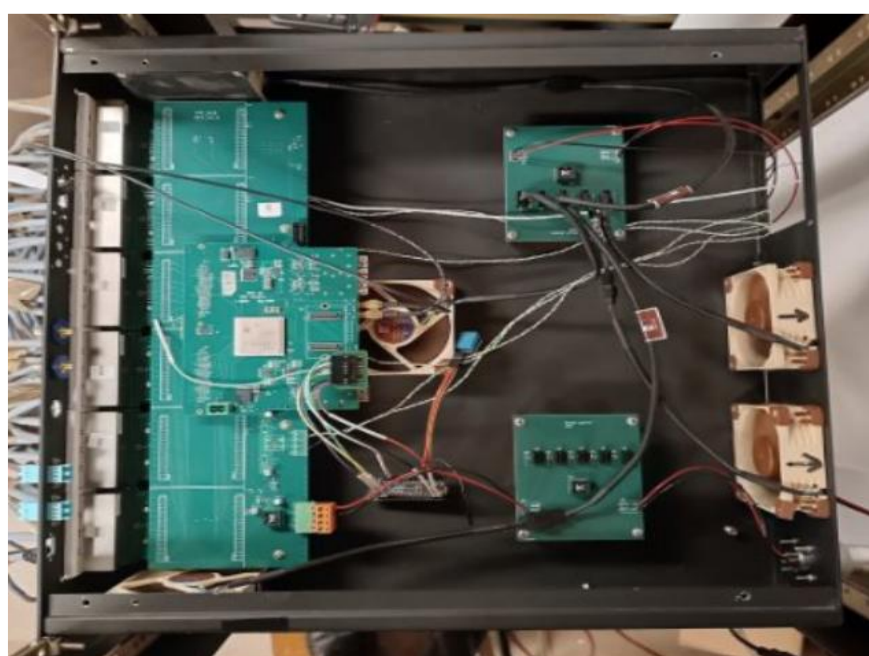
Fig: Setup for ESP32+Sensor+FPGA
