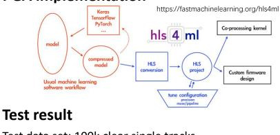
Test data set: 100k clear single tracksMLP structure: 24-48-32-16-8-1CLK: 400MHzFPGA: XCKU060Dead time: 4 clksLatency: 30clks
