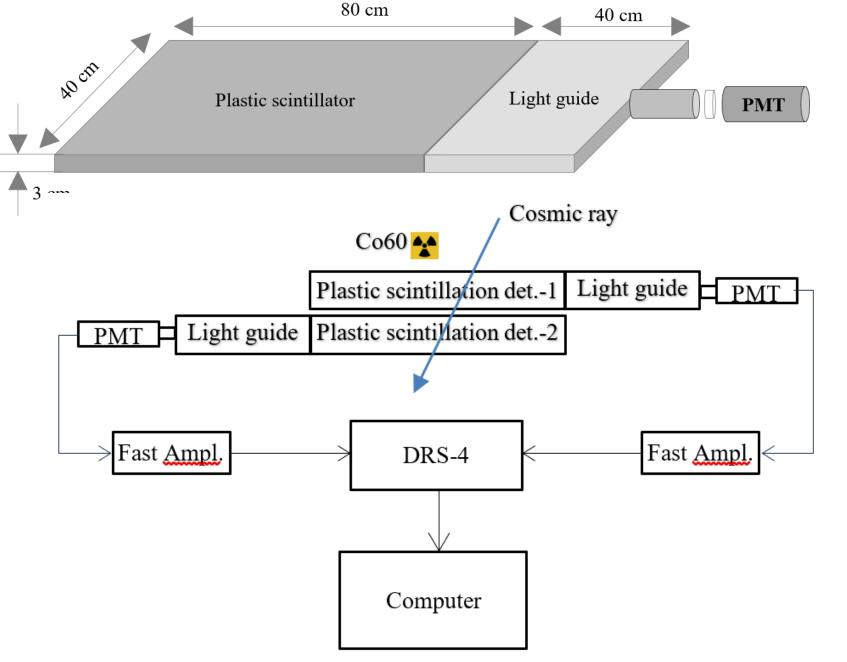
Output of the PMT is amplified by a fast amplifier and recorded by the digitizer of DRS-4 [3] in the form of basic waveforms.
