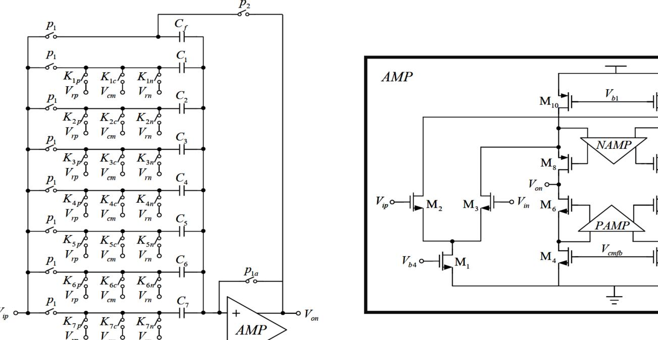
Figure 3. Structure of the first-stage MDAC circuit on one side
